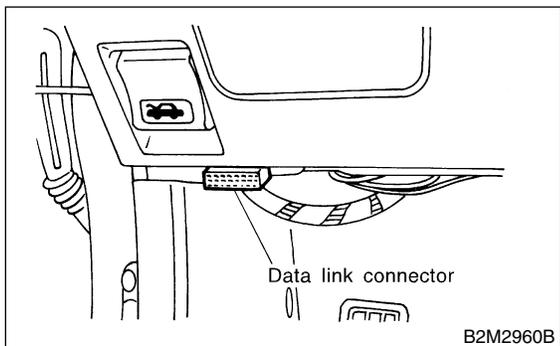
3) Using the OBD-II general scan tool, call up diagnostic trouble code(s) and freeze frame data.
