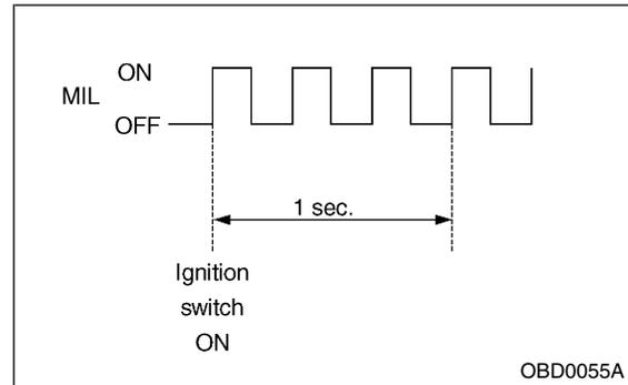
2) After starting the engine, the MIL goes out. If it does not, either the engine or the emission control system is malfunctioning.
