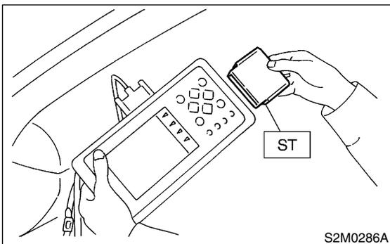
4) Connect test mode connector at the lower portion of instrument panel (on the driver's side), to the side of the center console box.
